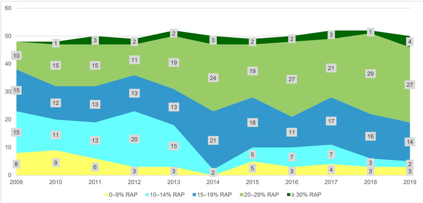
Figure 8: Number of States at Different Average Percentage of RAP Used in HMA/WMA Mixtures, 2009–2019
