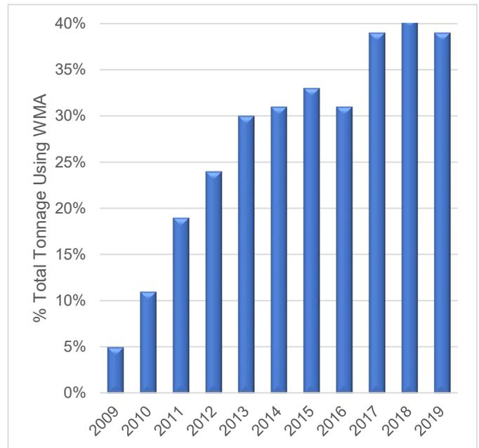
**Figure 15: Percent Total Tonnage Produced Using WMA Technologies**
