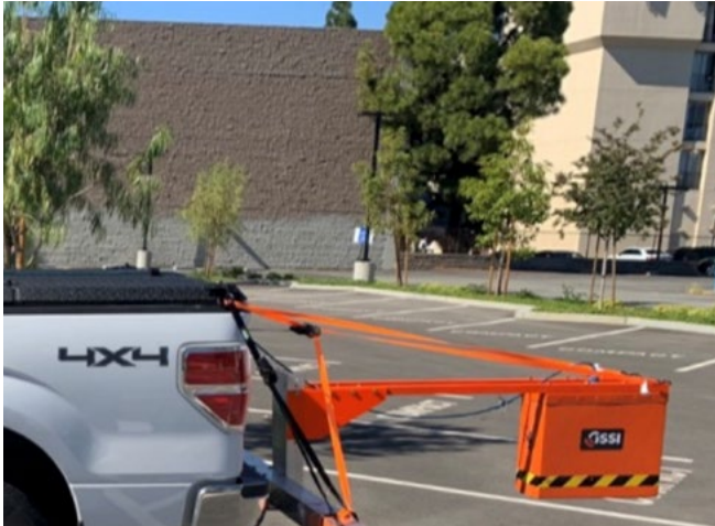
Figure 6. Example of GPR equipment.
