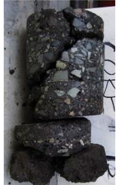
c. Stripping and delamination.
