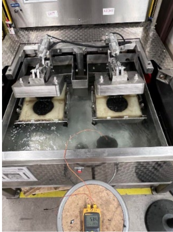
Figure 12. Dummy Sample with Temperature Probe When Conditioning Compacted Asphalt Mixtures in HWT Test Water Bath
