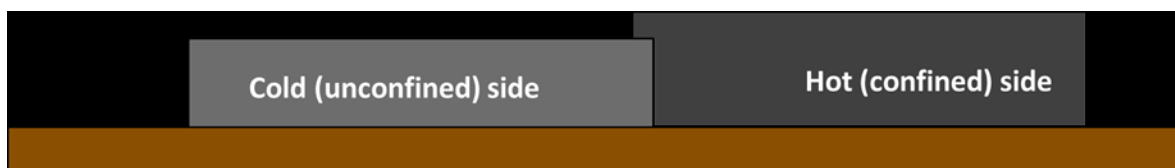
Figure 125. Common Terms for Transverse and Longitudinal Joints
