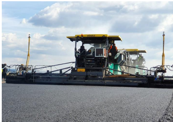
Figure 107. Dual Receivers on a Paver
