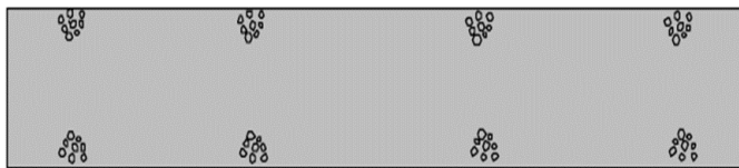
Figure 151. Examples of Truck-End Segregation
