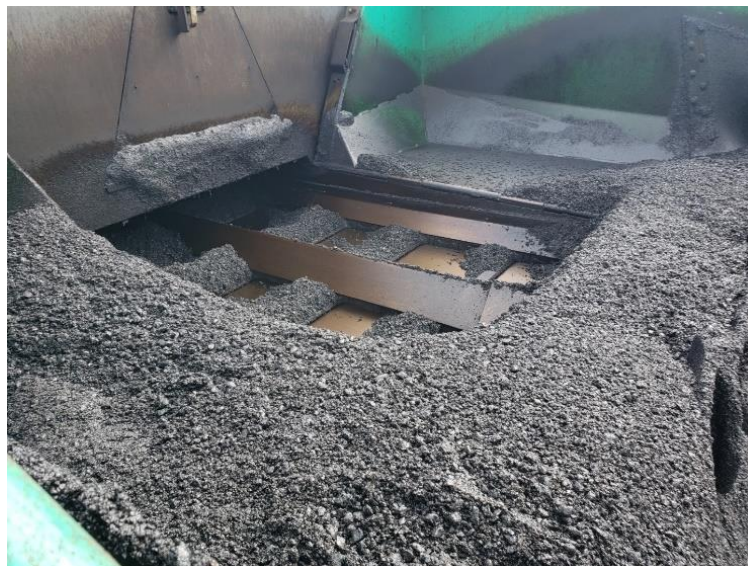
Figure 89. Poorly Managed Paver Hopper
