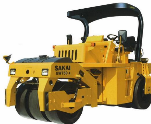
Figure 118. Vibratory Pneumatic Rubber-Tired Roller
