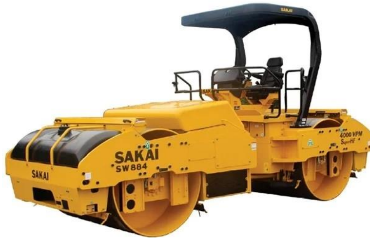
Figure 120. Double-Drum Vibratory Roller Equipped with IC Technology
