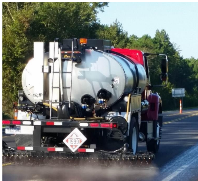
Figure 63. Distributor Applying Tack Coat
