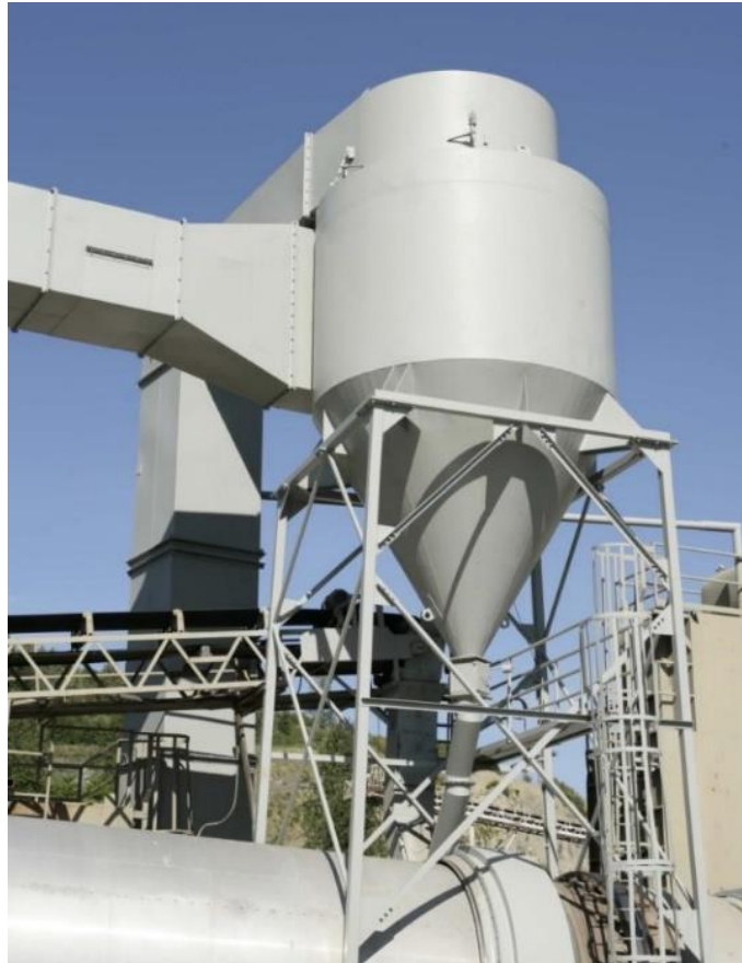
Figure 49. Cyclone Collector Returning Coarse Fines to the Dryer
