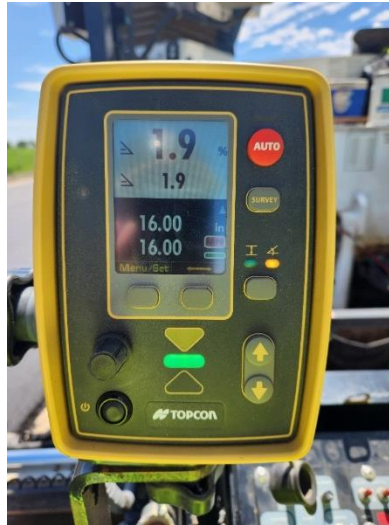
Figure 106. A Modern Cross Slope Controller
