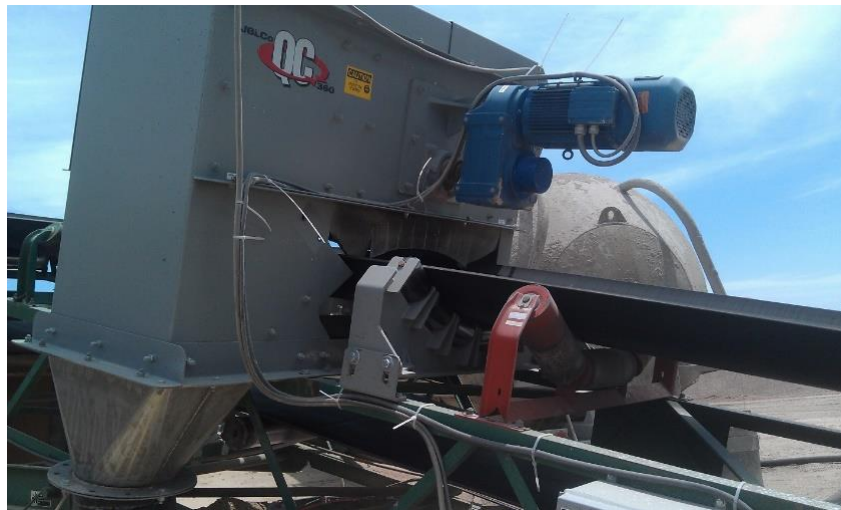
Figure 43. Conveyor Belt Sampling Device
