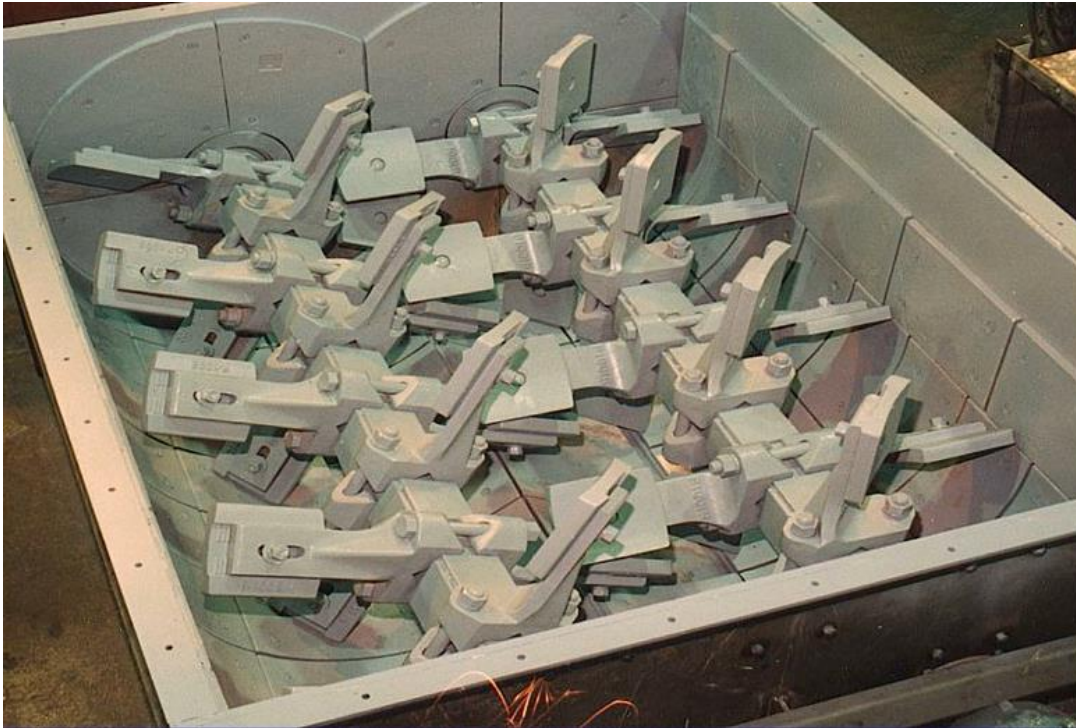
Figure 39. Batch Plant Pugmill
