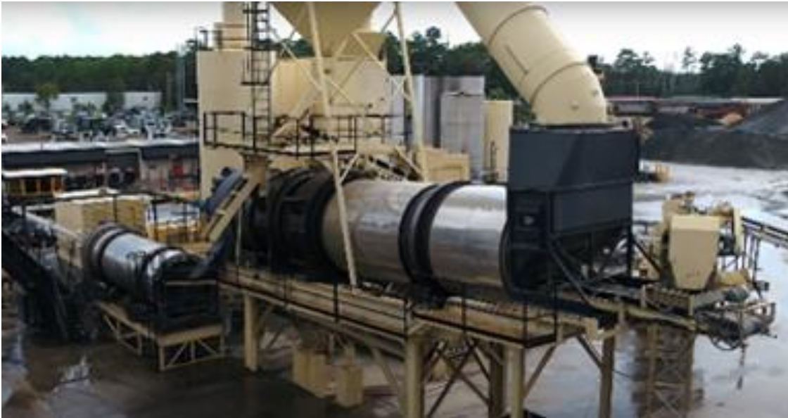
Figure 29. Typical Batch Plant Dryer
