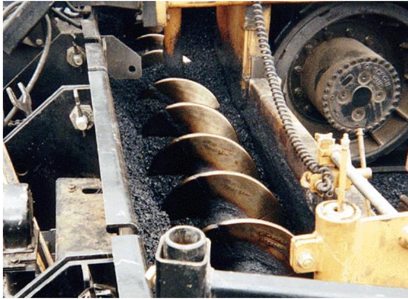
Figure 158. Proper Mix Height in the Auger Box
