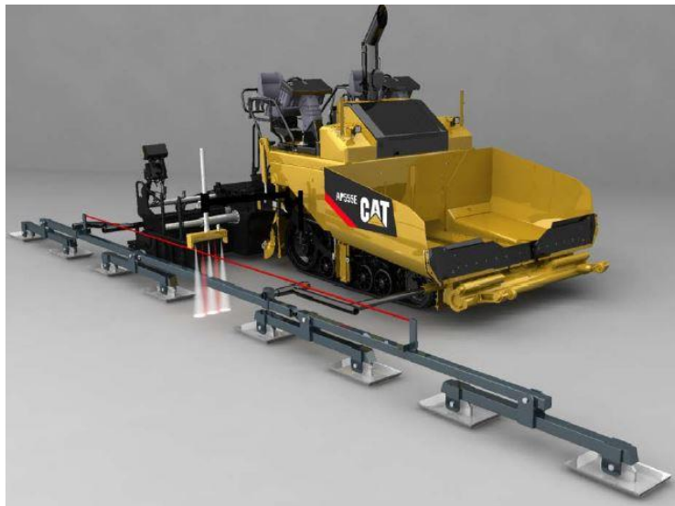
Figure 101. Floating-Beam Grade Reference
