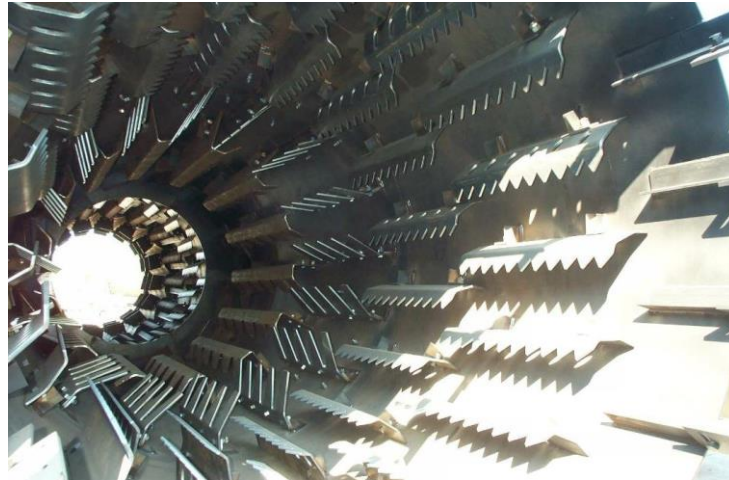
Figure 31. Different Types of Dryer Flights
