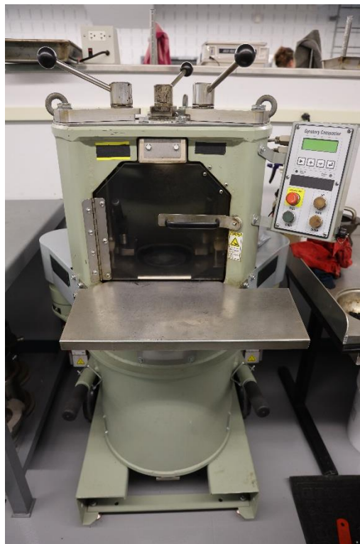
Figure 20. Superpave® Gyratory Compactor
