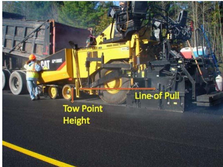
Figure 94. Tow Point and Line of Pull
