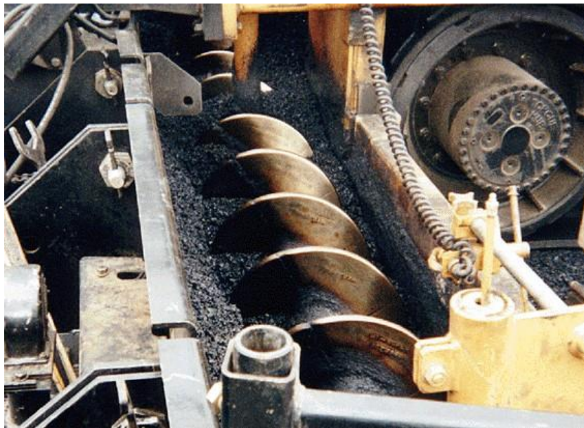
Figure 85. Uniform Head of Material at Axle Height
