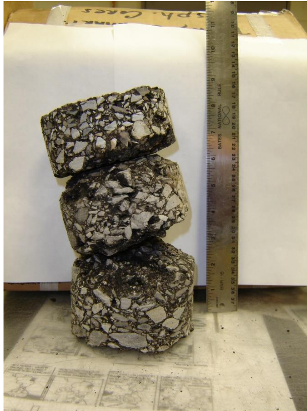
Figure 16. Stripping at the Lift Interface
