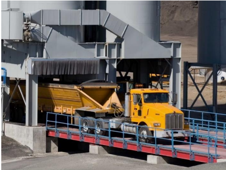
Figure 55. Truck Scale Under Storage Bins
