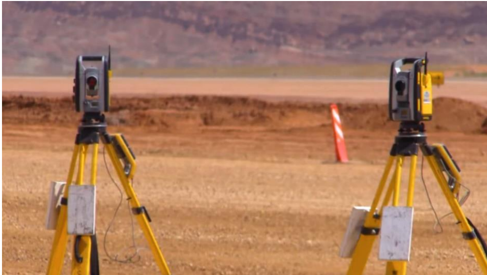
Figure 108. Universal Total Station Tracking Paver
