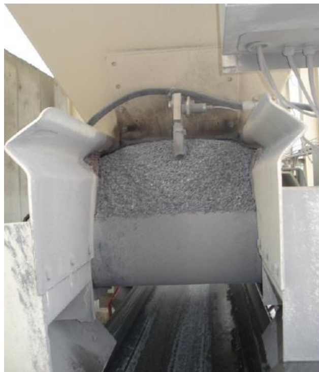
Figure 26. Bin Feed Aggregate Sensor
