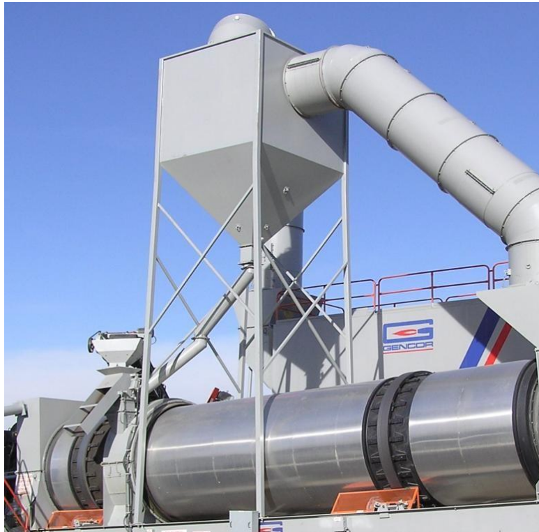
Figure 48. Knockout Box Returning Coarse Fines to the Dryer
