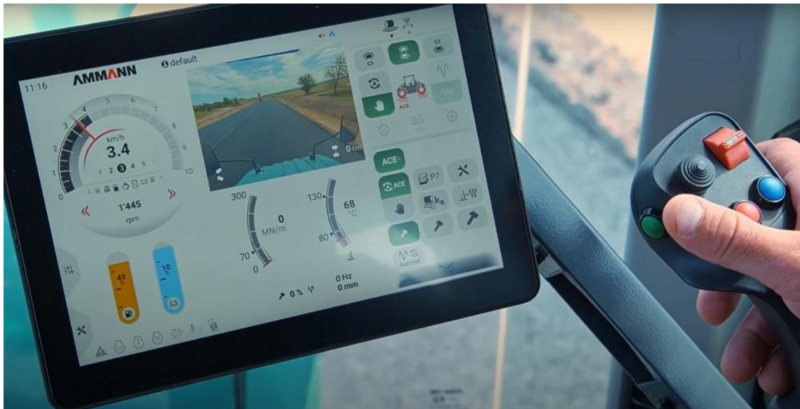
Figure 119. Roller Equipped with IC Technology
