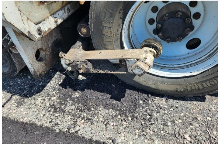
Figure 80. Truck Hitch on Front of Paver
