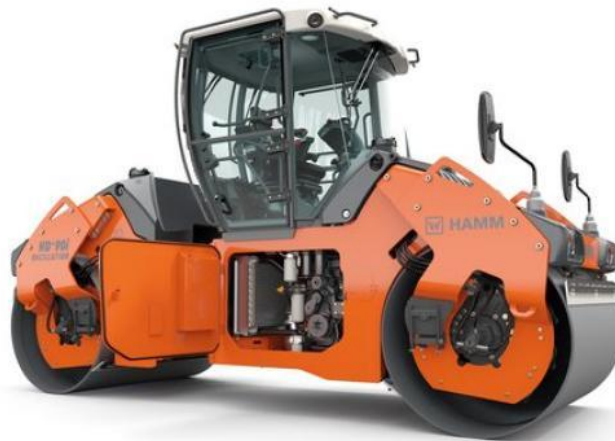
Figure 116. Double Drum Oscillatory Roller
