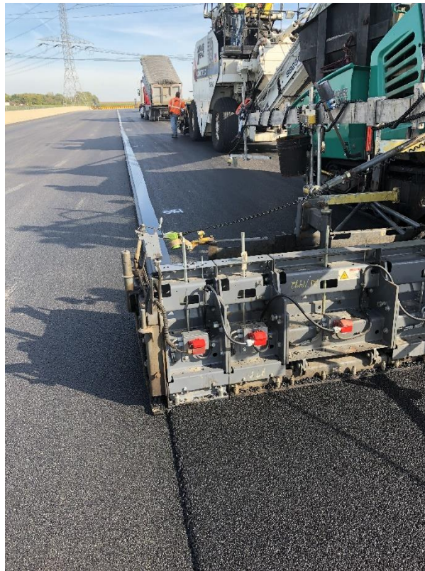
Figure 92. Fixed-Width Screed with Vibratory Bolt-On Extensions
