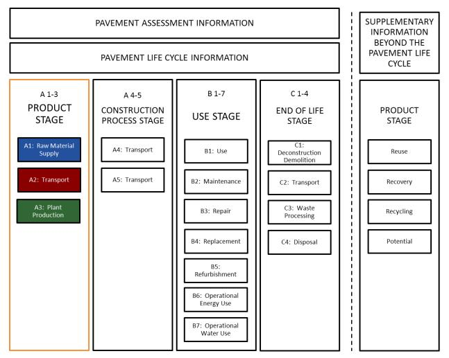
Figure 1. Diagram of designations of modular information used for life cycle assessments for pavements (adapted from CEN EN 15978:2011). This PCR's boundary is in the box outlined in orange, covering Modules A1–A3.
