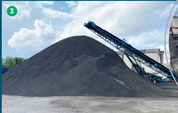
Figures 3 and 4. RAP stockpiles built using ramps help reduce moisture accumulation prior to processing RAP
