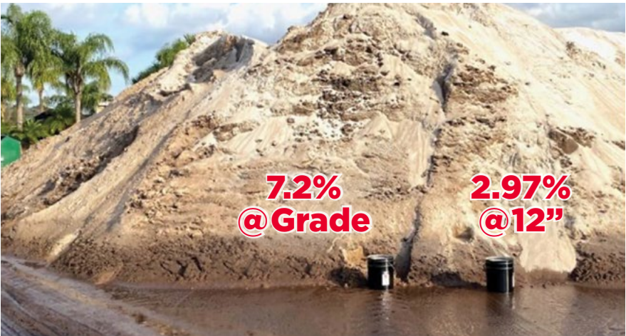
Figure 2. Natural sand stockpile moisture measurements
