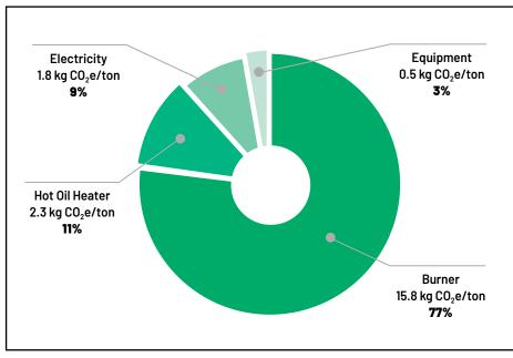
**Figure 6.** Mix production related GHG emissions (A3) for a typical asphalt plant with grid-supplied electricity that consumes natural gas for the burner and hot oil heater and diesel fuel for mobile equipment. Data inputs are provided in Appendix A. The sum of individual unit processes does not equal the A3 total of 20.5 due to rounding effects.
