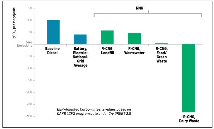
Figure 13. Life cycle carbon intensity (CI) values for CNG as a transportation fuel sourced renewable sources (R-CNG). R-CNG feedstocks have low or even negative CI scores because they capture emissions that would otherwise be released to the atmosphere. From NGVAmerica (2019).
