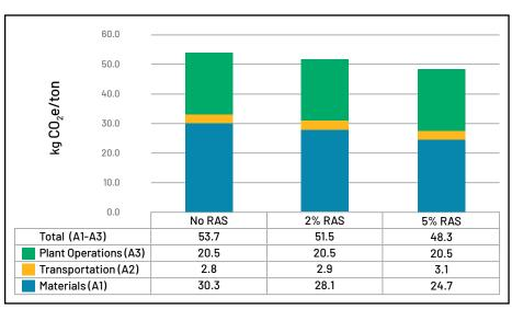
**Figure 9.** Impact of RAS on cradle-to-gate (A1-A3) emissions of an asphalt mixture. Total asphalt binder content for each mix is 5%. RAS is assumed to have a 20% asphalt binder content and to offset the virgin binder content accordingly (e.g., a mix with 5% RAS would have a virgin binder content of 4% and a recycled binder content of 1%). Units in the data table are in kg  $CO_2e$ /ton of mix. The sum of individual life cycle stages may not equal the total due to rounding effects.
