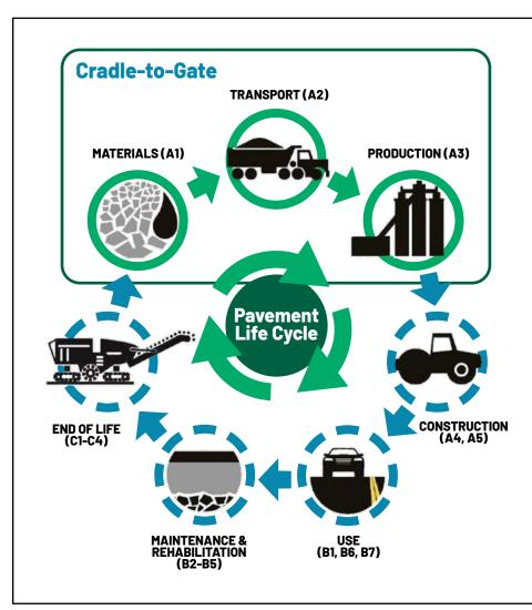
Figure 1. Key stages of the asphalt pavement life cycle with reference to the ISO 21930 life cycle information modules.
