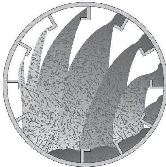
Figure 30. Uniform Veil of Aggregate in Dryer
