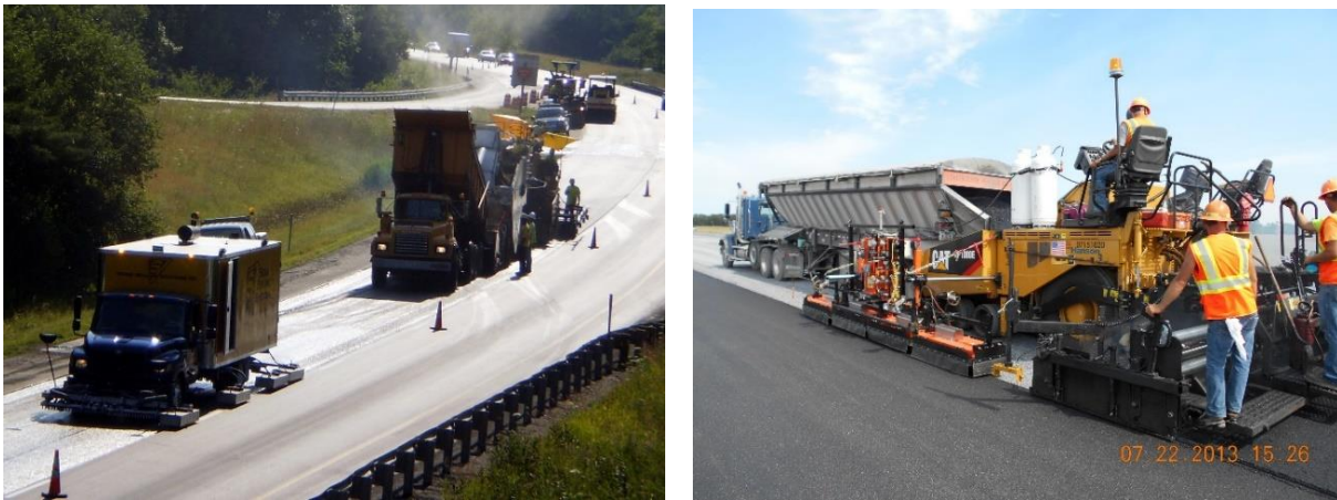
Figure 147. Joint Heaters: Self-Contained (left) and Paver-Mounted (right)
