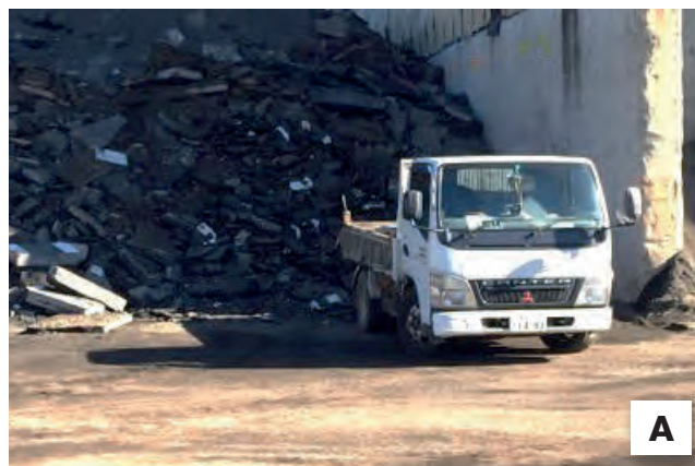
Figure 2-3. Photos from the Taisei Rotec Tokyo Aomi Asphalt Mixing Plant and Tokyo Rinkai Recycling Center. (A) Receiving recyclable pavement waste; (B) Enclosed recycling facility; (C) Primary roller crusher; (D) Indoor processing equipment; (E) Fractionated RAP, –13 to 5 mm on left, –5 mm on right; (F) Samples of coarse and fine fractionated RAP.
