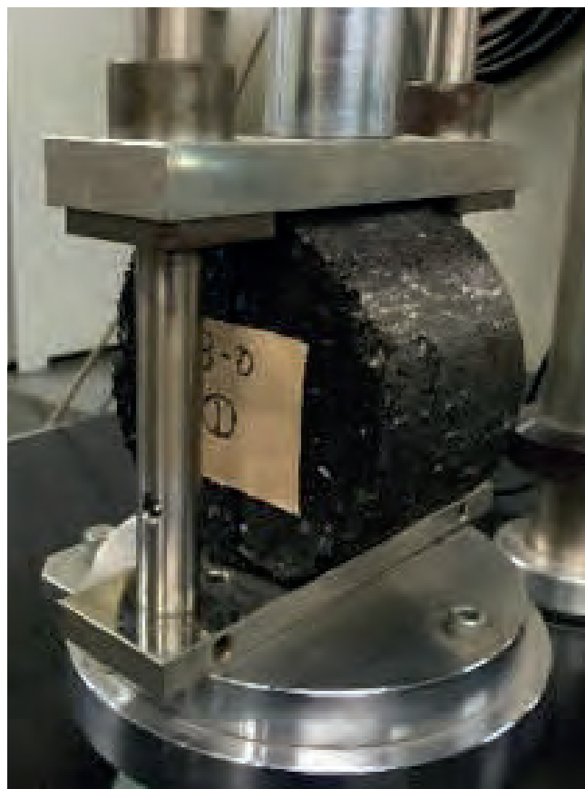
Figure 2-4. Indirect tensile strength test used for evaluating RAP and mixes containing RAP.
