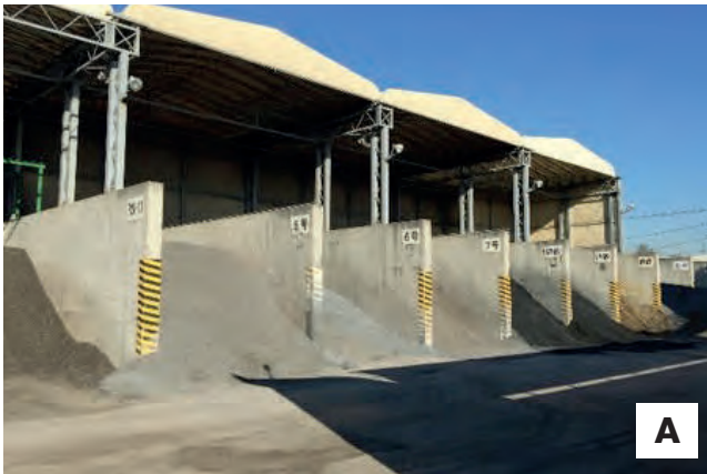
Figure 2-12. Photos from the Maeda Road Construction Co. Ltd. asphalt plant in Kawasaki, Kanagawa Prefecture. (A) Aggregate storage bins; (B) Aggregate cold feed bins; (C) RAP cold feed bins for two size fractions; and (D) Parallel-flow RAP dryer with natural gas burner in foreground.
