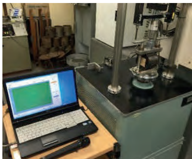
Figure 2-4. Indirect tensile strength test used for evaluating RAP and mixes containing RAP.
