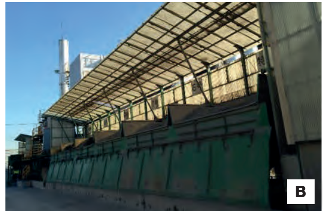
Figure 2-12. Photos from the Maeda Road Construction Co. Ltd. asphalt plant in Kawasaki, Kanagawa Prefecture. (A) Aggregate storage bins; (B) Aggregate cold feed bins; (C) RAP cold feed bins for two size fractions; and (D) Parallel-flow RAP dryer with natural gas burner in foreground.
