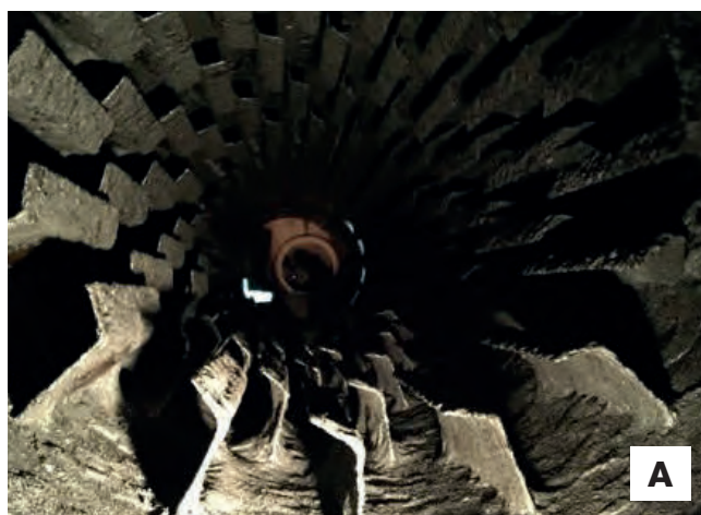
Figure 2-13. (A) Inside of RAP dryer; (B) Pugmill for mixing hot RAP with rejuvenator; (C) Batch hopper conveyor to move rejuvenated hot RAP to surge bin; (D) Downward view of a counter-flow aggregate dryer; (E) Aggregate hot bins above weigh hopper; and (F) Plant view of three RAP surge bins on the left and four hot-mix silos on the right.
