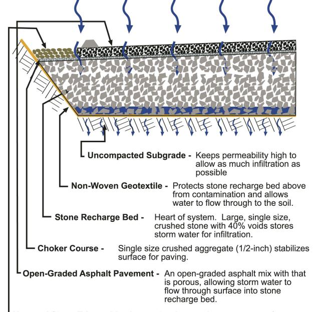
**Unpaved Stone Edge -** A backup system in case the pavement surface should ever become sealed. Storm water can flow off pavement surface to stone edge and into stone recharge bed.
