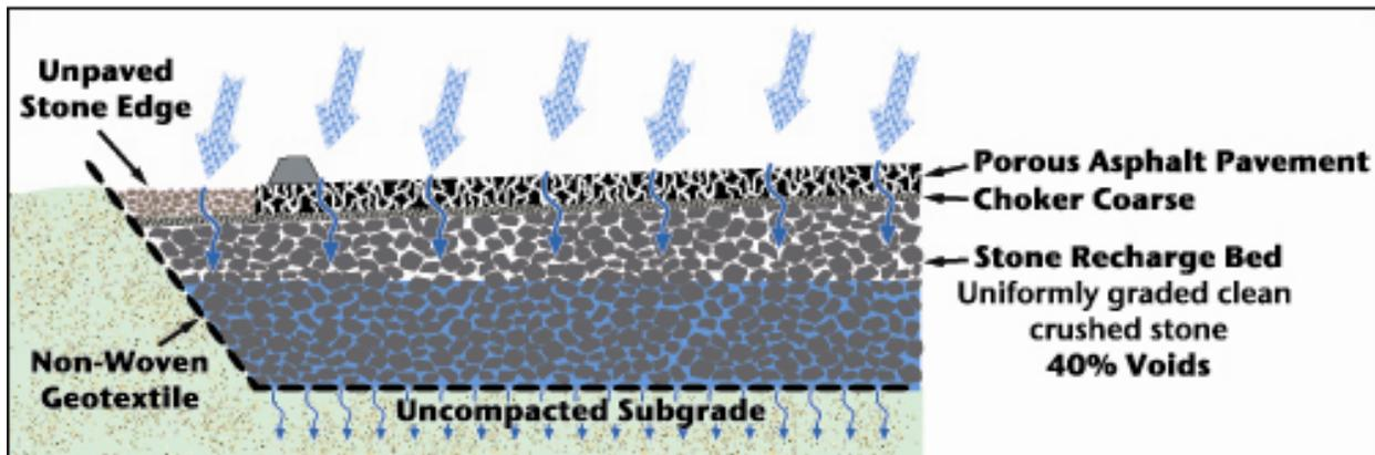
Figure 2. Schematic of a porous pavement
