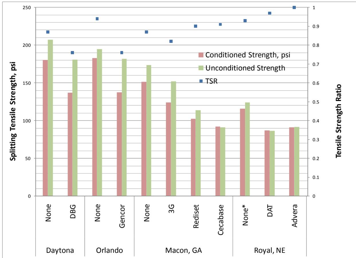
**FIGURE 3 Tensile Strength Ratio Results**
