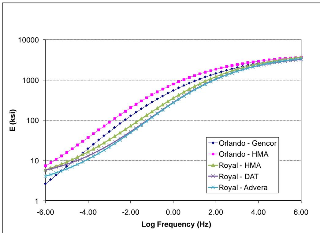
**FIGURE 1 Unconfined Dynamic Modulus Results.**
