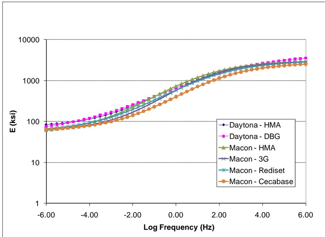
**FIGURE 2 Confined Dynamic Modulus Results.**
