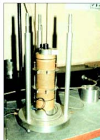
Figure 2. Photograph of Triaxial Soil Sample.
