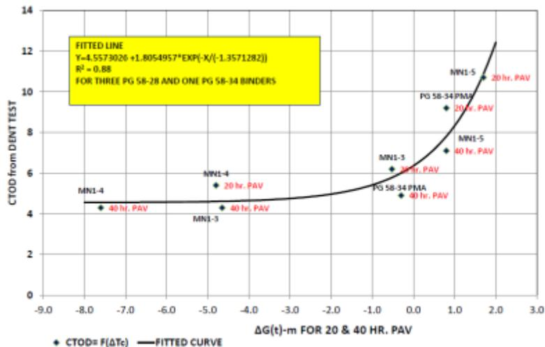
Figure 5: CTOD from DENT vs.  $\Delta T_c$
