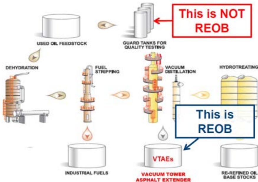
Figure 4: Identification of REOB in manufacturing process (supplied by Safety-Kleen)
