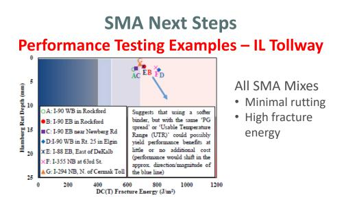
Figure 8. Performance-space diagram of test sections.
