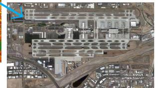
The biggest heat island in the Phoenix, Ariz., metropolitan area is Phoenix Sky Harbor International Airport, with its thick concrete runways. North Scottsdale Road, which is made of asphalt, is demonstrably cooler in this NASA ASTER Night Surface Temperature image.
